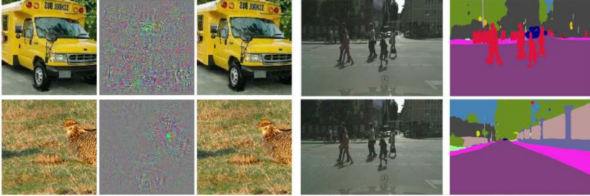
Figure 2.2.: Adversarial examples generated using the L-BFGS approach. Left: input sample x , middle: noise pattern p and right: resulting input. Courtesy of [SZS + 13]
